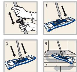
In this way, all the loose dust is fully removed from the floor in a very simple manner.
